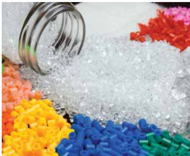
Plastic resins used in the manufacture of consumer items such as plastic bottles and plastic bags.
